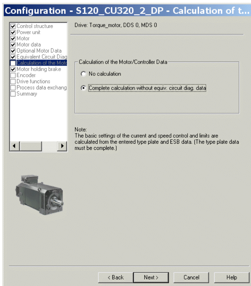
Figure 3-76 Screen form for calculating the motor/controller data
